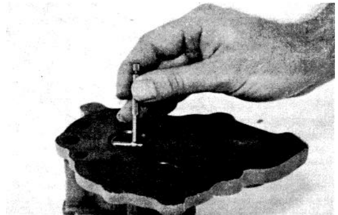
Fig. 7-7. Measure The Inside Diameter Of The Bushings.
