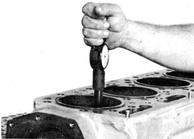
Fig. 14-12. Measure The Bore Of The Liner.
