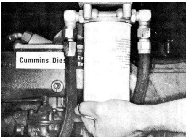
Fig. 2-19, (VI1909). Changing "spin-on" type fuel filter
