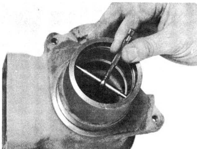
Fig. 8-23 (N10866). Measure The Bore In The Housing.
