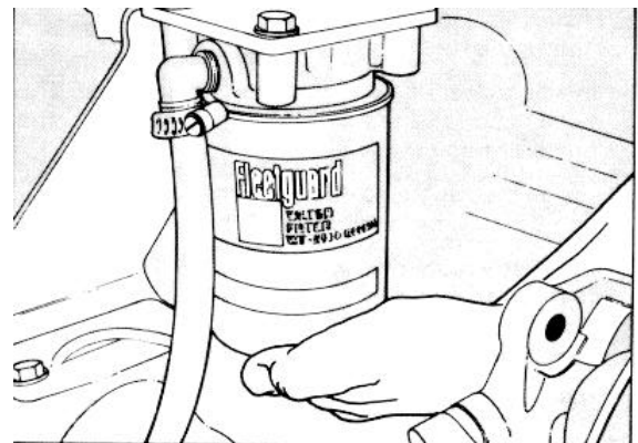
Fig. 2-23, (OM1023L). Installing DCA water filter cartridge
