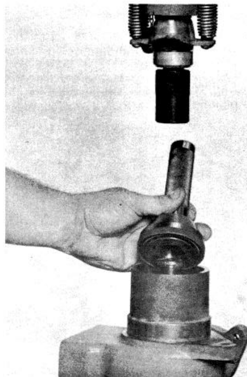
Fig. 8-29 (N10872). Install The Seal Into The Housing
