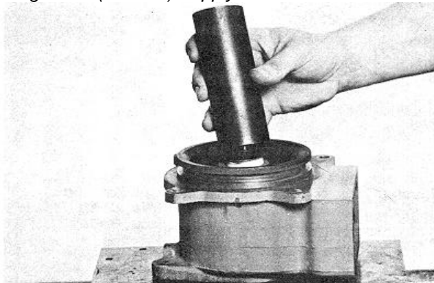
Fig. 8-30 (N10853). Apply Loctite Onto The Seal.
