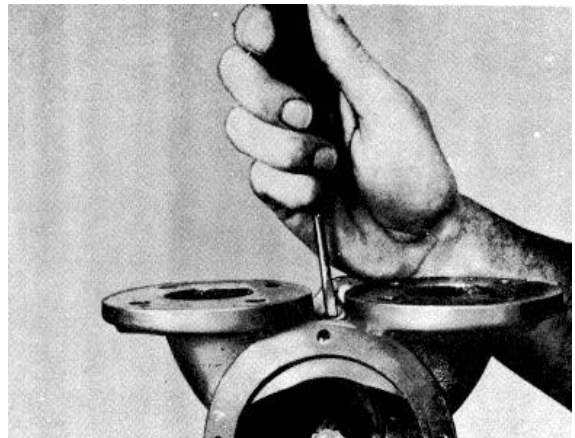
Fig. 8-59 (N20807). Install The Cam And Wear Plate.
