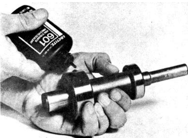
Fig. 8-27 (N10870). Apply Loctite Onto The Bearings.
