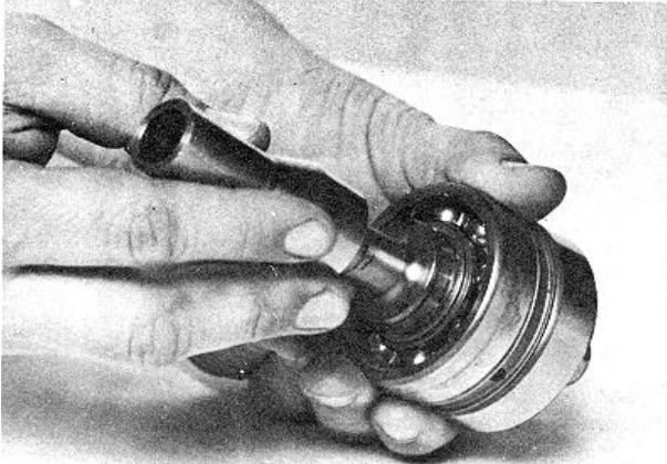
Fig. 8-48 (N10889). Install The Pilot For The Oil Seal Onto The Shaft.
