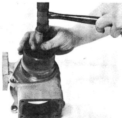
Fig. 8-17 (N10860). Remove The Oil Seal From The Housing.
