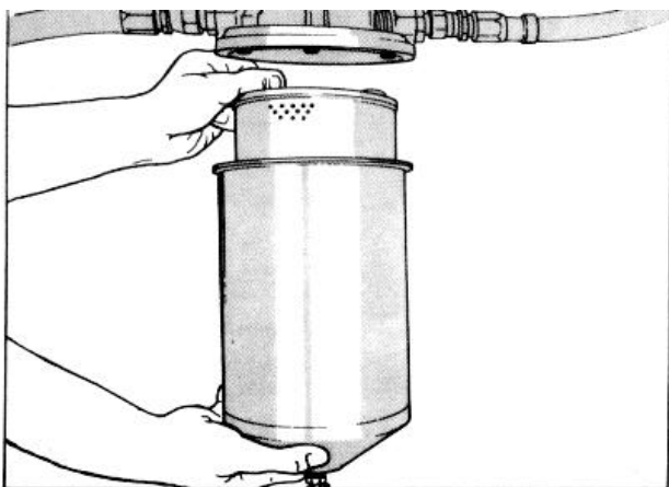
Fig. 2-20, (OM1021L). Installing replaceable fuel filter element
