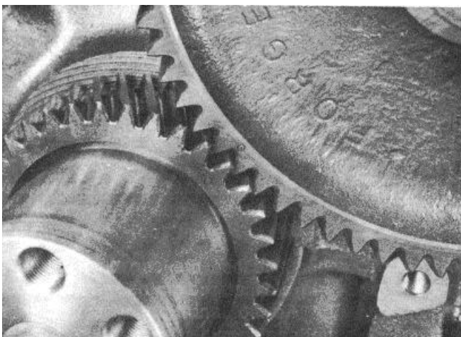
Fig. 14-22. Align The Timing Marks On The Camshaft Gear And Crankshaft Gear.
